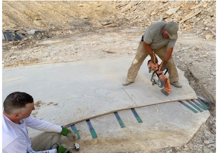
Figure 4. The owner of Warfield Fossil Quarries, Rick Hebdon, cuts out a fish fossil while APS member Shane looks on. Steel shims hammered along the edge of the slab force the layers to split along a single plane. Photo: Keith Mychaluk.
