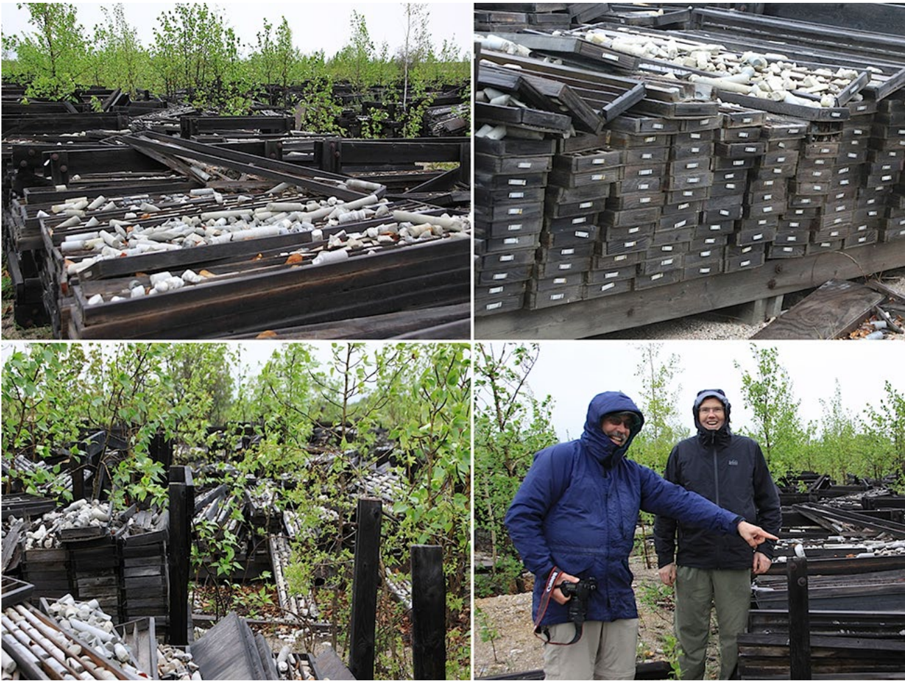
Figure 6. Top left: Cominco left its core boxes behind, having abandoned the mining lease in 2001. I presume the company felt no liabilities could result from leaving the boxes. Top right: Cores were cut in a systematic fashion to determine where the best lead (galena) and zinc (sphalerite) ore could be found. Each core was examined by geologists and then stored in these wooden boxes. Half cores indicate sampling for ore quality. Each box was labelled with an aluminum tag recording the pit, core sequence and core lengths. Lower left: Nature is reclaiming the area with poplar trees. The boxes, some hardly touched in 2006, are now well pilfered by the human element. Lower right: The traditional pose when a neat item is found. In this case Wayne is pointing out a calcite crystal making up this piece of core. Wayne and Don are bundled up because it was only 6° C with a wind chill that made it -7° C this day! My hands were so cold after a couple of hours exposure, that I could only peel half of my orange.
